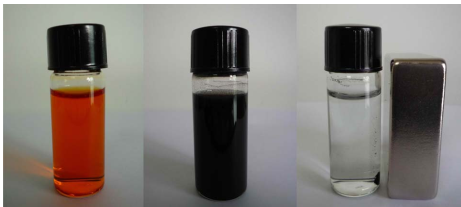
Figure 10. Photographs of the initial MO solution ( 100 \text{ mg L}^{-1} , left), the solution after mixing with HPGCM-Ni-900 (middle), and the solution after removal of MO dyes by a magnet (right). [Color figure can be viewed in the online issue, which is available at wileyonlinelibrary.com .]
